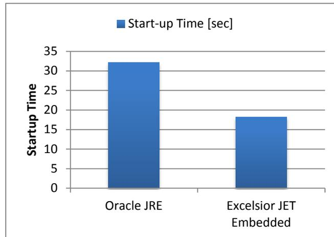
**Figure 2, Embedded application start-up time**
