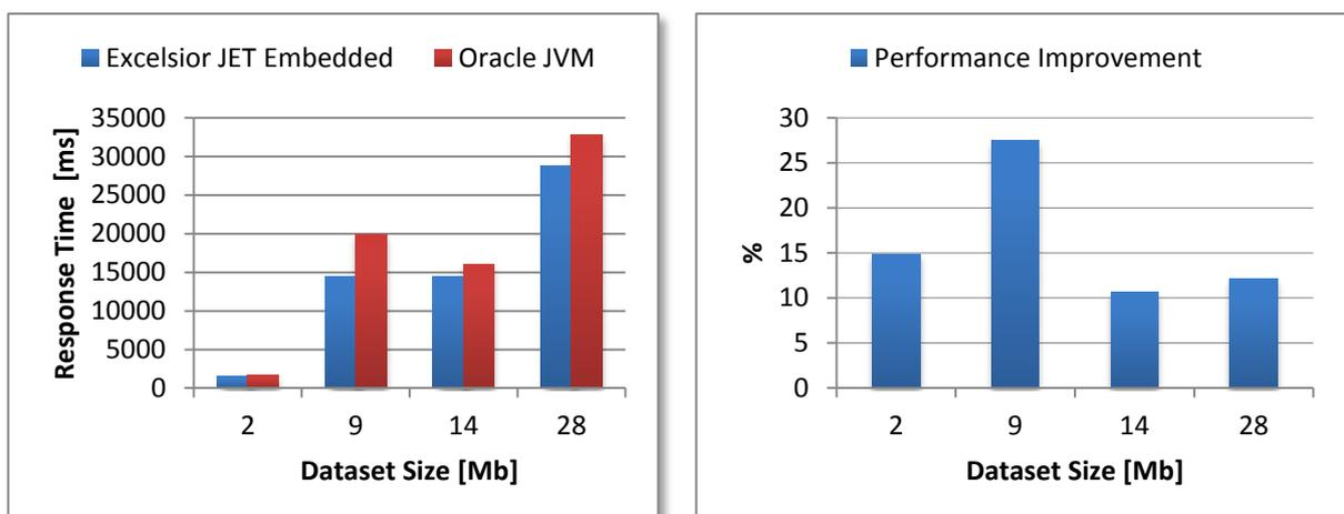
**Figure 3, Embedded application performance times for various dataset sizes**
