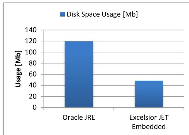
**Figure 4, Embedded application disk space usage**
